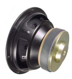
The magnet system features a vented pole piece in order to avoid over/under pressure behind the dust cap (mechanical damping) when the cone is moving. The cone is made from air-dried paper. Normally when making paper cones, the water is pressed out of the cone simply because letting it air-dry is way too time consuming.
